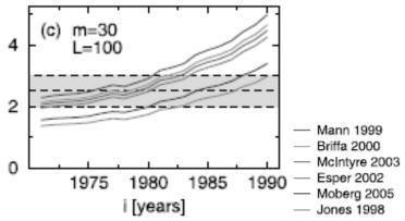
The result is given in the diagram; the curves are all the same, but they differ in scale because of the unit of different standard deviations derived from the reconstructions given at the figure caption. The horizontal dashed lines mark 2, 2.5 and 3 standard deviations. Two standard deviations correspond to a risk of false rejection of the null hypothesis of 2.5%.
