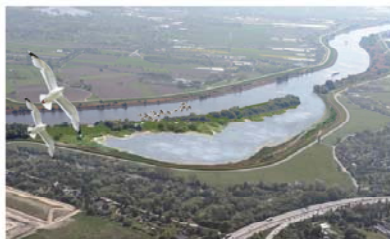
Fig. 2: (Montage) Newly created shallow water areas in the upper estuary will not only benefit the sediment regime, but could – depending on size and design – also be used as flooding areas or polders to reduce storm surge peak levels.
